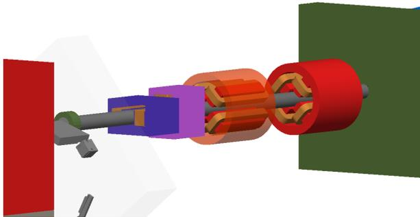
Figure 2: Detailed model of the energy degrader and the beginning of the rotating gantry. A cylindrical 4D-Scoring is placed on the Q1G quadrupole. The last radial bin fits the iron external geometry of the magnet. On the figure, the external geometry of Q1G was removed and the last bin of the scoring mesh was highlighted in red.
