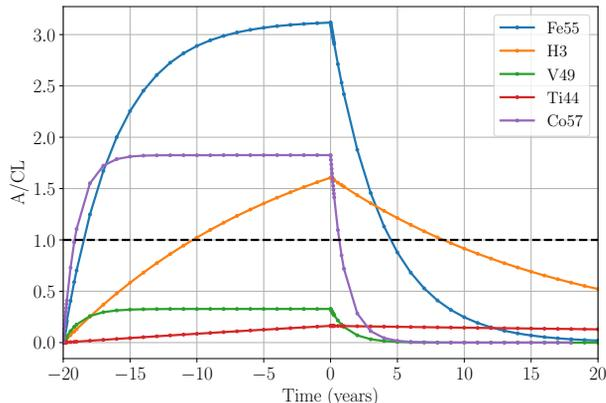
Figure 6: Evolution of the clearance index with time of the most radioactive part of the Q1G external structure following the main radioactive nuclides, other than  $^{54}\text{Mn}$ .
