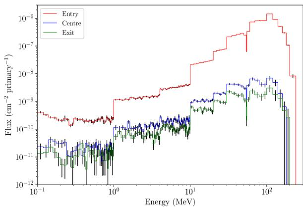
Figure 3: Differential secondary neutron fluence (left) and proton fluence (right) extracted from the Q1G external structure using the BDSIM 4D Scoring feature. The fluence has been extracted at the entry, the centre and the exit of the Q1G outer structure. The energy bins follow the CCFE-709 and CCFE-162 energy group structures, respectively.
