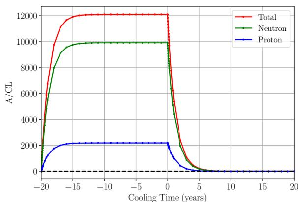
Figure 5: Evolution of the clearance index with time of the most radioactive part of the Q1G external structure following the incident particle type.
