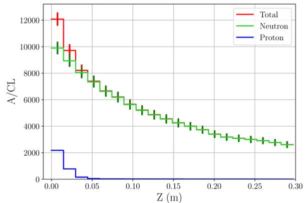
Figure 4: Evolution of the clearance index along with the thickness of the Q1G external structure. The clearance indexes related to the neutron and proton activation are represented in green and blue, while the total is represented in red.
