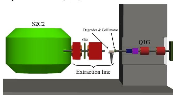
Figure 1: BDSIM model of the vault extraction line and its shielding. The S2C2 and the energy degradation system are shown. The concrete shielding wall separating the cyclotron vault from the treatment area is visible, with the beamline elements fit through a cylindrical cut.
