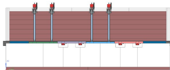
Figure 2: Novel multi-jaw collimator design candidate Elevation cross section. Beam travel is left to right.
