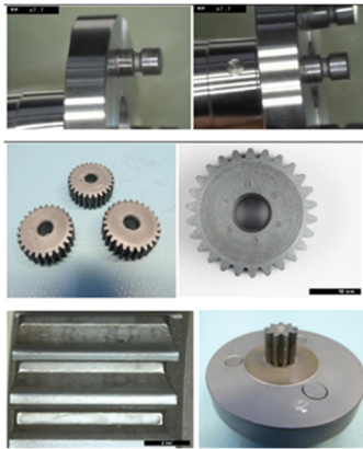
Figure 4: The second stage of gear box did not show significant damage.
