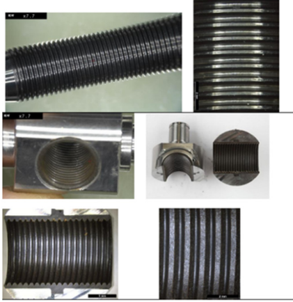
Figure 3: Pictures of Titanium shaft and TECASIN traveling nut. No visible wearing after 2-month longevity test.
