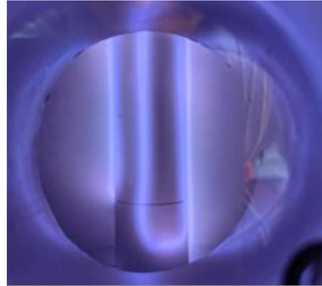
Figure 5: The bottom turn-around region of the niobium radial magnetron while actively depositing material with a HiPIMS plasma.
