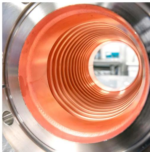
Figure 3: Coated LCLS-II bellows section using 1" magnetron design.
