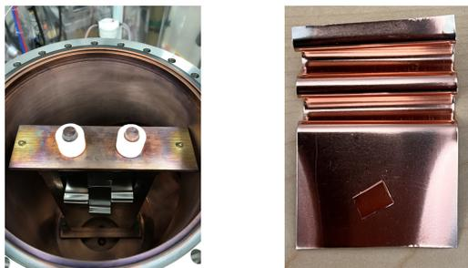
Figure 2: Stand-in volume for CEBAF waveguide (left). Example test coupon used for characterizing film uniformity (right).
