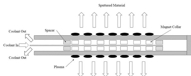
Figure 1: Diagram of 0.5" outer diameter magnetron for coating CEBAF waveguides. Magnet pack creates distinct erosion patterns around each stack of magnets.
