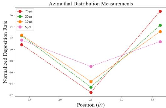
Figure 4: Deposition rate measurements at various negative pulse conditions. Measurements were taken directly in front of each magnetron and at a half-way point between them.
