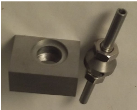
Figure 3: Photographs of cathode and anode of magnetron SPS with active cooling.
