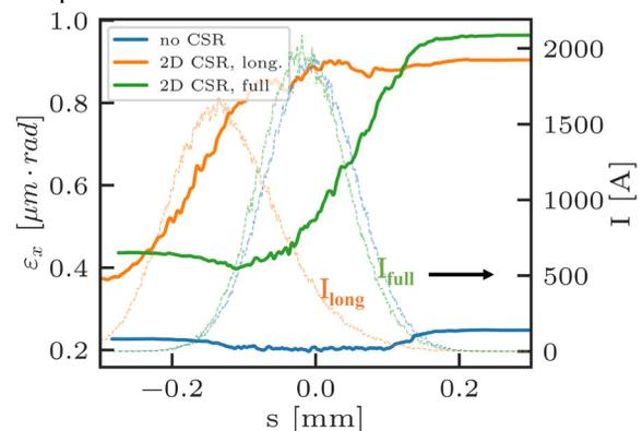
Figure 1: Beam slice remittances (left) and current profiles (right) without CSR, or with only longitudinal or full 2D steady-state CSR effect.
