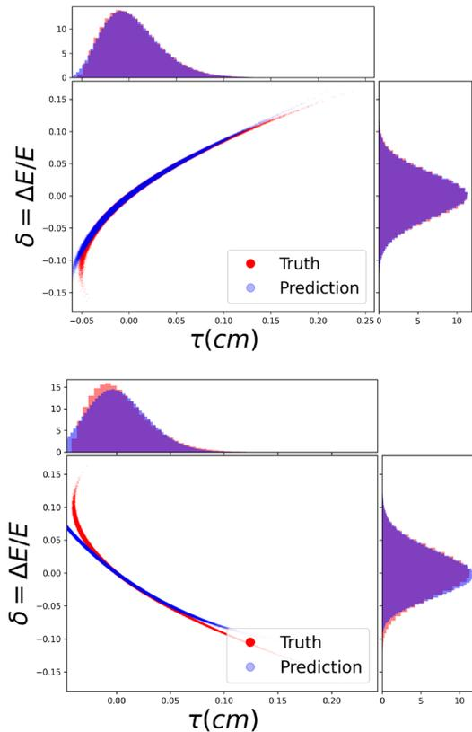
Figure 2: Preliminary HenonNet model prediction of the longitudinal phase space ( $\delta = \Delta E/E$ ,  $\tau$ : bunch length in cm) of electron beams with 10% initial energy chirp after a chicane compressor with length: (top) 2x longer, (bottom) same as the beam in the training data.
