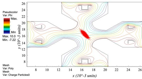
Figure 3: Visualization of a trapped beam of  $^{24}\text{Mg}^+$  in the CRFQ using VSim.
