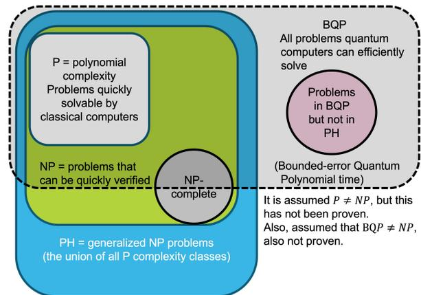
Figure 1: An Euler diagram illustrating the relationships of different complexity classes for classical and quantum computing. This is an active area of research, so this diagram is only meant to generally show how different classes of problems fit into either a classical or quantum computing universe [10].
