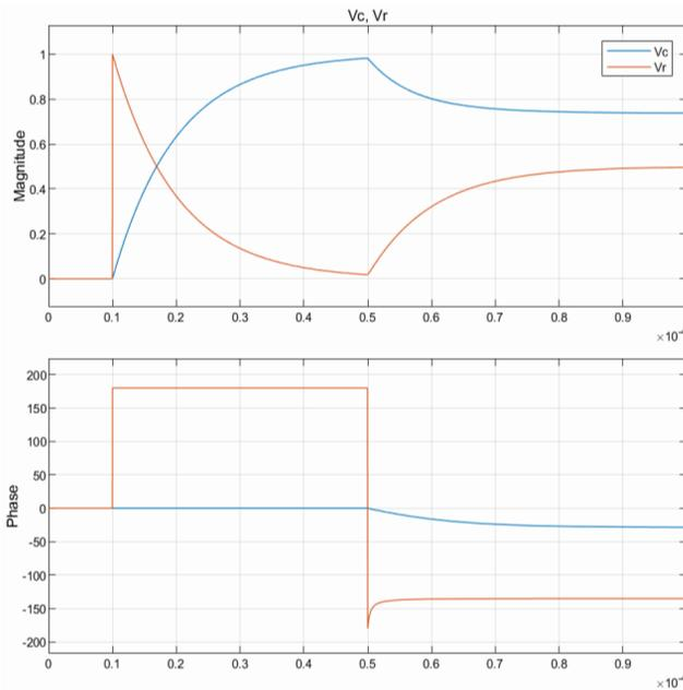
Figure 4: Response of critically-coupled cavity with beam loading.
