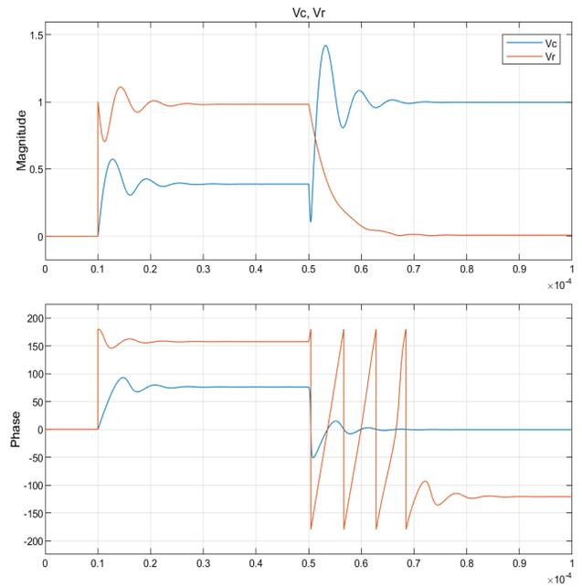
Figure 5: Overcoupled and detuned response.
