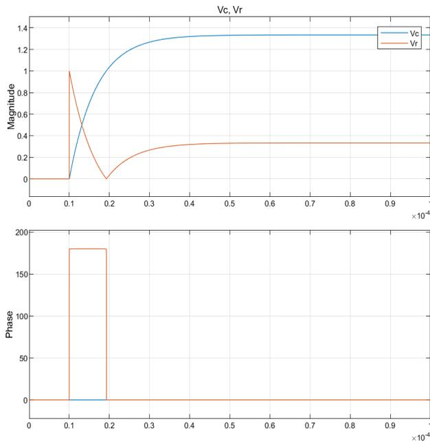
Figure 3: Response of overcoupled cavity.
