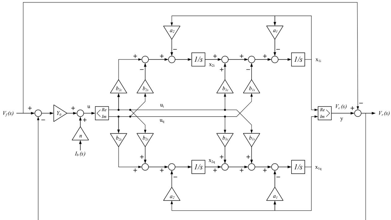
Figure 2: State-space realization block diagram of loaded cavity in second companion form.
