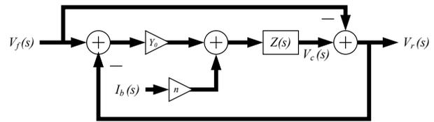
Figure 1: Operational block diagram of line/beam/cavity interactions.
