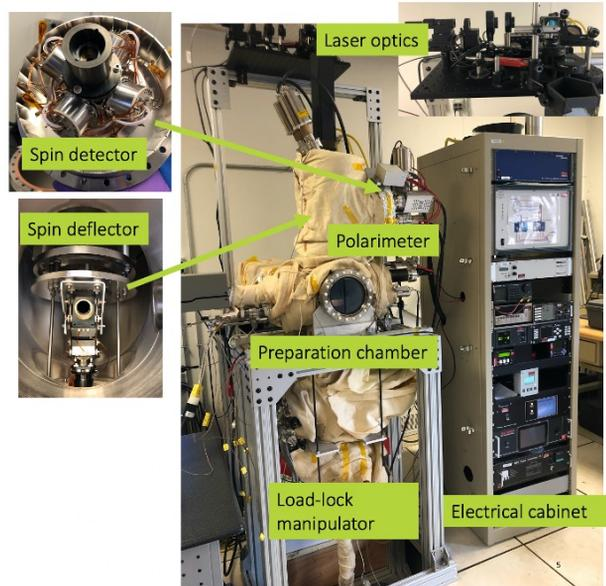
Figure 4: The picture of the Mott polarimeter system at BNL, which is used for activation of photocathode and measurement of the QE and ESP.
