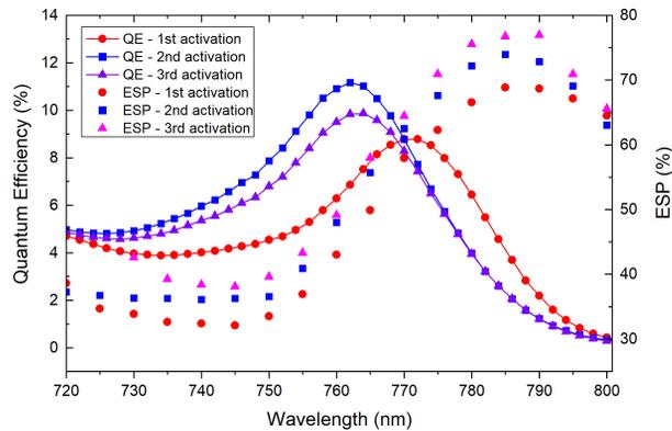
Figure 6: The QE and electron-spin polarization for the GaAs/GaAsP superlattice DBR photocathode as a function of the wavelength, measured at the edge of the wafer.
