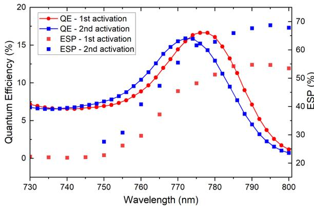
Figure 5: The QE and electron-spin polarization for the GaAs/GaAsP superlattice DBR photocathode as a function of the wavelength, measured at the center of the wafer.
