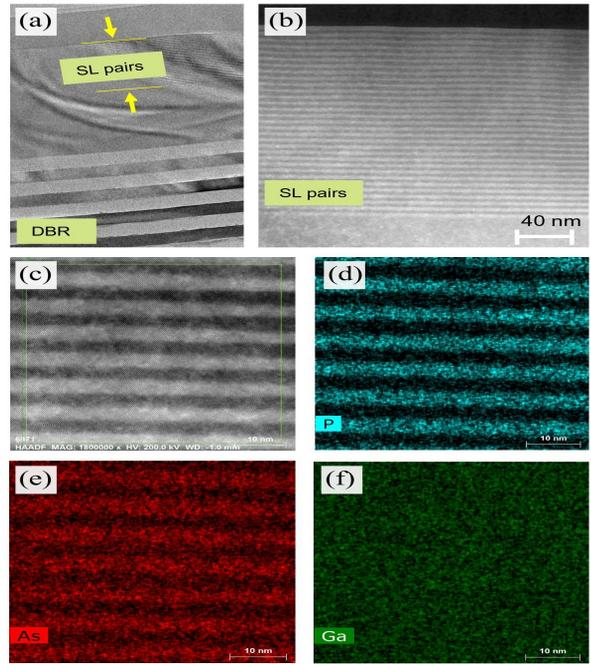
Figure 3: (a) Cross sectional TEM images of SL-DBR GaAs showing both SL and DBR pairs. Bend contours are visible which are associated with the bent sample with respect to the incident electron beam. The number of DBR-pairs was 10. (b) STEM image showing uniform SL-pairs (c) TEM image of a few SL-pairs, (d) EDS map of P, (e) EDS map of As, and (f) EDS map of Ga.
