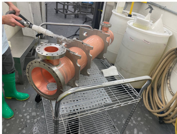
Figure 8: Micro90 detergent cleaning of the body.
