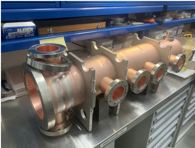
Figure 4: The kicker cavity after all the ports have been vacuum brazed in the body.
