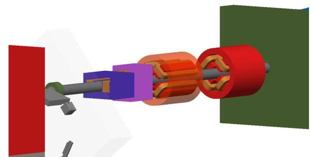
**Figure 2:** Detailed model of the energy degrader and the beginning of the rotating gantry. A cylindrical 4D-Scoring is placed on the Q1G quadrupole. The last radial bin fits the iron external geometry of the magnet. On the figure, the external geometry of Q1G was removed and the last bin of the scoring mesh was highlighted in red.
