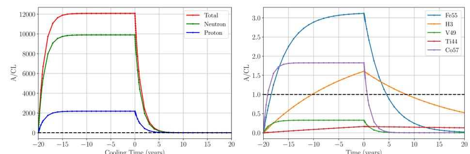
**Figure 5:** Evolution of the clearance index with time of the most radioactive part of the Q1G external structure following the incident particle (left) and the main radioactive nuclides, other than  $^{54}\text{Mn}$  (right).
