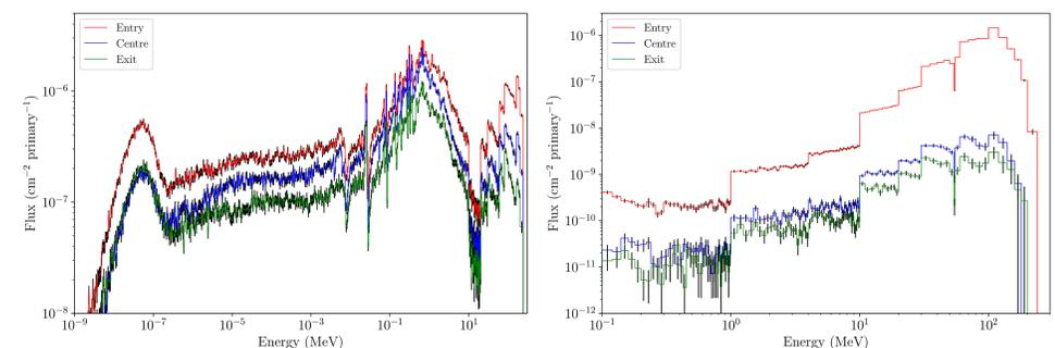
**Figure 3:** Differential secondary neutron fluence (left) and proton fluence (right) extracted from the Q1G external structure using the BDSIM 4D Scoring feature. The fluence has been extracted at the entry, the centre and the exit of the Q1G outer structure. The energy bins follow the CCFE-709 and CCFE-162 energy group structures, respectively.
