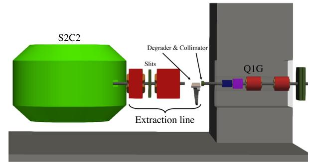
**Figure 1:** BDSIM model of the vault extraction line and its shielding. The superconducting synchro-cyclotron (S2C2) and the energy degradation system are shown. The concrete shielding wall separating the cyclotron vault from the treatment area is visible, with the beamline elements fit through a cylindrical cut.
