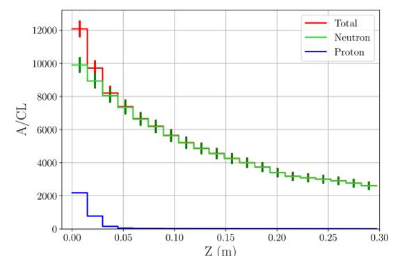
**Figure 4:** Evolution of the clearance index along with the thickness of the Q1G external structure. The clearance indexes related to the neutron and proton activation are represented in green and blue, while the total is represented in red.
