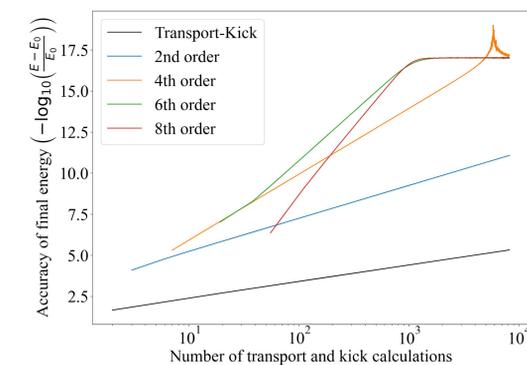
Convergence for different integrator orders with increasing slicing of the lens.
