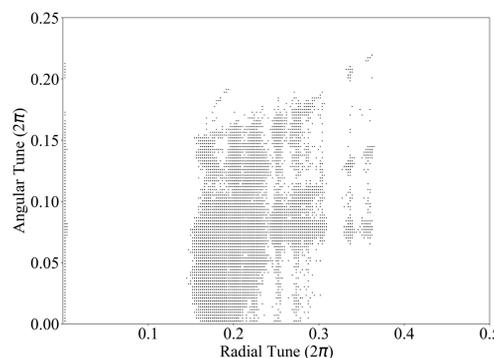
Tune spread from a strong ( $k = 1.076\text{m}^{-1}$ ) lens for 430 turns.
