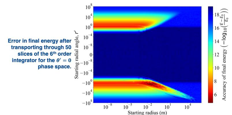
Error in final energy after transporting through 50 slices of the 6th order integrator for the  $\theta' = 0$  phase space.
