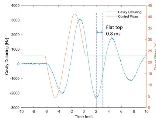
Figure 5: 160 Hz single cycle sine wave and the cavity detuning response.
