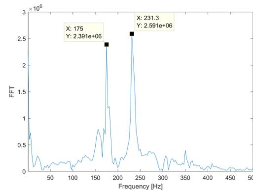
Figure 4: FFT of the cavity detuning from the simulated LFD pulse
