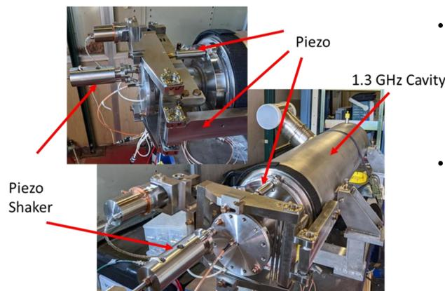
Figure 1: Setup of LFD simulation with 1.3 GHz cavity. Two piezo capsules are used for resonance control and a piezo (denoted as shaker) is used to simulate the LFD.
