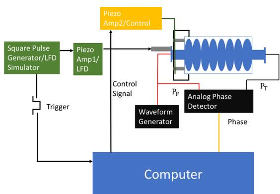
Figure 2: Schematic of signals used to measure the cavity frequency and for resonance control. A square wave pulse generator was used to simulate the LFD pulse and to trigger the control.
