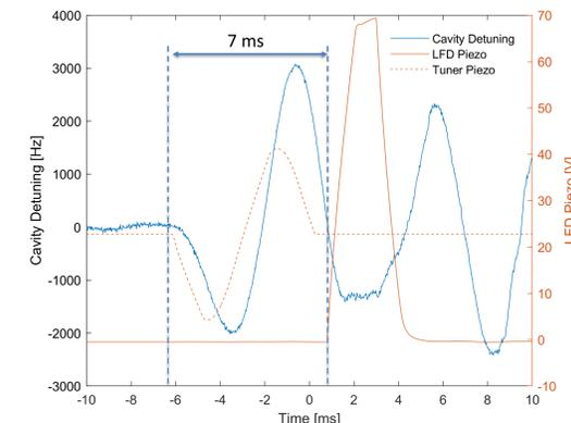
Figure 6: Control pulse which results in a flat cavity detuning. A sine wave of 160 Hz with a delay of 7 ms was used.
