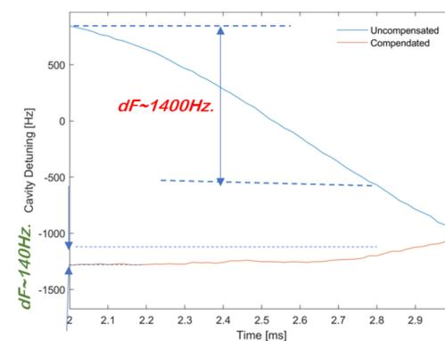
Figure 7: Comparison of cavity detuning with piezo control on and off. The results show that when the LFD pulse is compensated the cavity detuning is decreased by a factor of 10.
