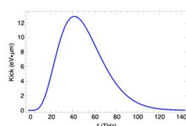
The energy kick, generated by one proton in the CEC kicker section. The longitudinal scale of the wake is  $\sim 3 \mu\text{m}$ , corresponding to the frequency bandwidth of interest of  $\sim 40 \text{ THz}$ .
