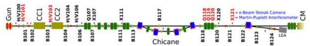
Diagnostics cross X121 (upstream of the SRF cyomodule) is presently equipped with an OTR screen, an Al-coated Si substrate, positioned at 45 degrees with respect to beam. Our Year-1 goal is to measure the single-bunch (45 MeV) OTR spectral energy density in the range of 0.9 – 2  $\mu\text{m}$ .
