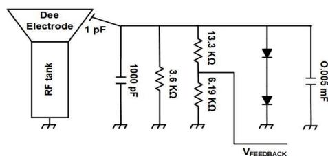
The probe consists of an isolated flush plate that faces the Dee electrode and has a 1 pF capacitance to the Dee electrode. A 1000 pF capacitor is connected to the plate to sample the RF, working as a 1/1000 divider. A resistor divider of 13.3 kΩ and 6.19 kΩ decreases the amplitude further, producing a feedback voltage,  $V_{FEEDBACK}$ , that is sent to the Dee voltage regulator.
