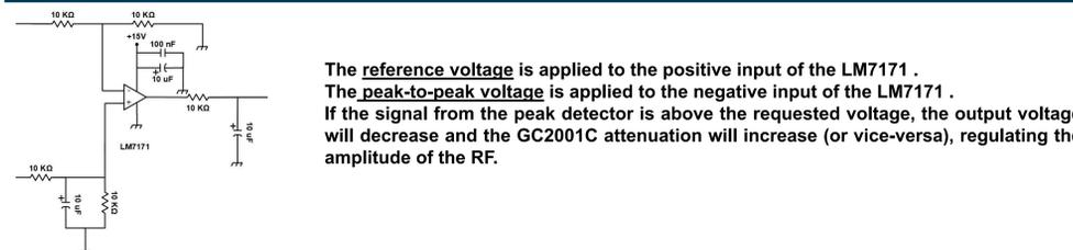
The **reference voltage** is applied to the positive input of the LM7171.
