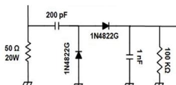
The peak-to-peak detector is a combination of two cascaded parts:
