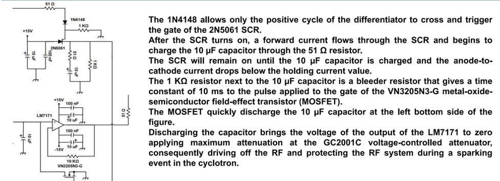
The 1N4148 allows only the positive cycle of the differentiator to cross and trigger the gate of the 2N5061 SCR.
