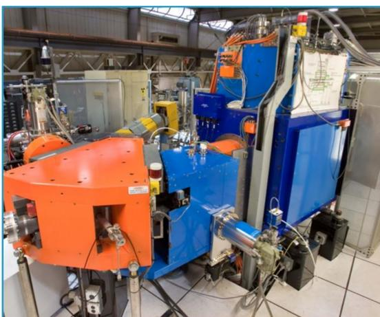
VENUS is a next generation superconducting ion source at Lawrence Berkeley National Laboratory that is used to feed the 88-inch Cyclotron with high-current and charged state ions to be accelerated.
