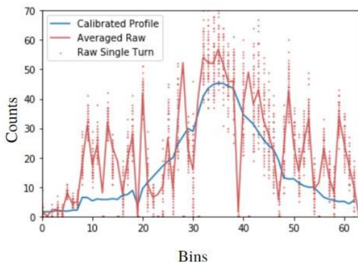
The above figure shows a vertical eIPM distribution taken at AGS injection. Raw profiles are in red, calibrated final profile is in blue. Bins with obviously incorrect results are considered 'dead' and are removed from the data. Since the measurement is taken at injection, tails are not due to 3<sup>rd</sup> order resonance.
