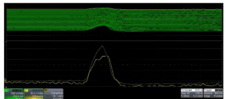
Longitudinal bunch lineshape varies little as the resonance saturates. This is true even in cases where particle loss is significant. This is consistent with crossing an adiabatic resonance.
