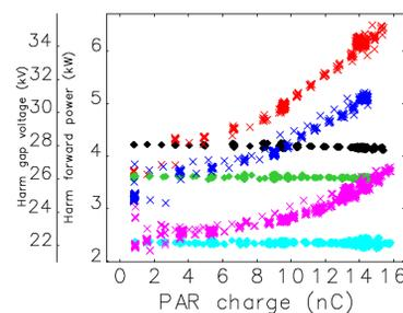
SSA amplifier forward power and gap voltage (22 kV, 26 kV, and 28 kV) as a function of bunch charge (8-kW limiter).
