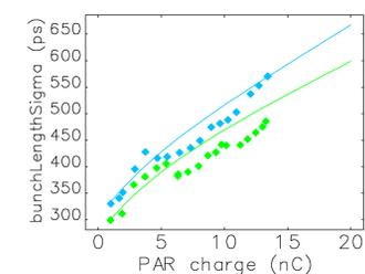
Comparison of measurements with predicted bunch lengths using Haisinski distributions (425 MeV, Z/n = 25 Ω, R = 1300 Ω).
