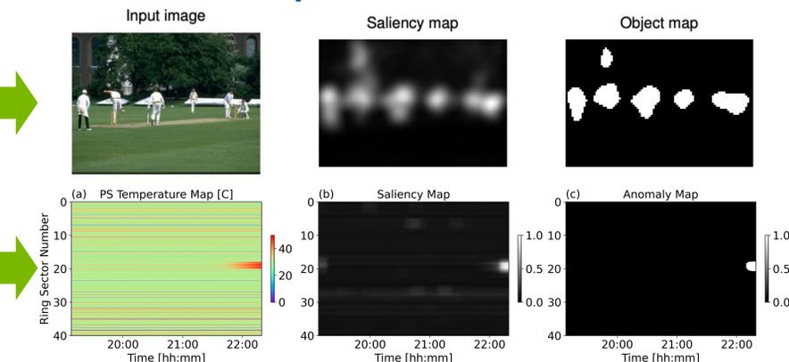
Autoencoder input: average PS temperatures in 40 sectors of the ring
