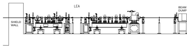
Figure 1: Schematic of the LEA beamline. Beam trajectory is from left to right.
