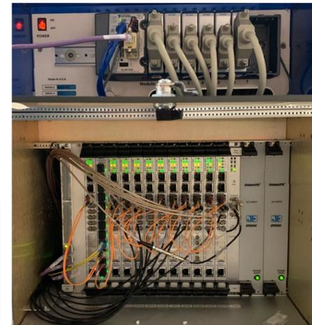
A custom cPCI/VPX architecture in one crate focus on beam-synchronized data acquisition. The cPCI side provides eight 6U cPCI slots for low cost per channel signal conditioning. One slot is usually reserved for a Micro Research Finland Event Receiver for crate timing information. The VPX side modularizes on a new VITA standard high-speed connector, with a switched PCI Express/Ethernet backplane fabric. The crate has six 3U VPX slots. It typically hosts up to five BittWare S43X
