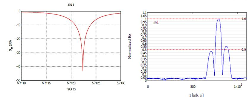
Fig. 5. Cold-test results for the first C-band  $a/\lambda=0.105$  cavity: S-parameter measurements (left), beadpull measurements of the electric field profile on-axis (right).
