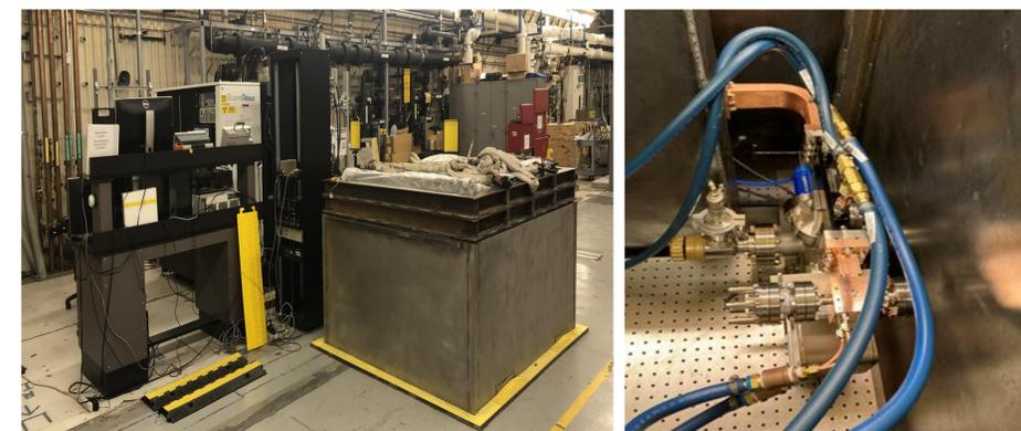
Fig. 1. (Left) LANL CERF-NM High Gradient test stand. (Right) Typical test setup with directional coupler, Faraday cup, water cooling and vacuum components
