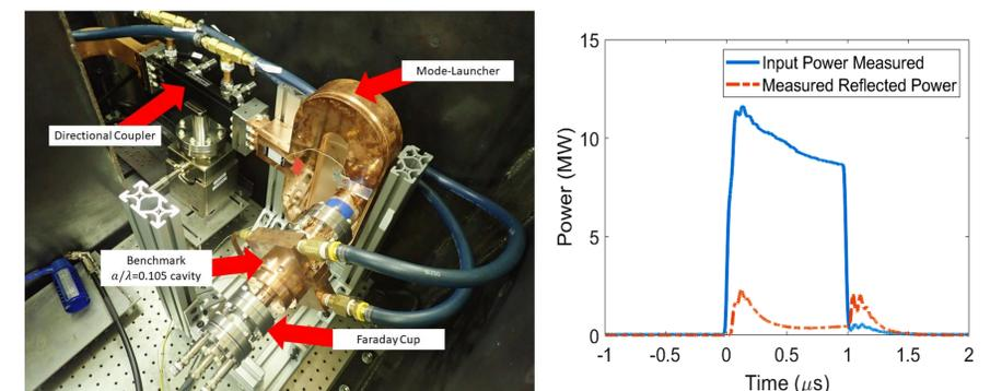
Fig. 6. (Left) High-gradient test setup for the benchmark  $a/\lambda = 0.105$  cavity. The mode-launcher is for on-axis coupling. The directional coupler is for pulsed power diagnostics and Faraday Cup attached to the end of cavity is for breakdown mapping. (Right) Pulse profile for breakdown mapping. The breakdown testing is being done now at a power level of 13MW.
