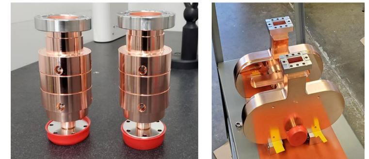
Fig. 4. LANL-fabricated benchmark  $a/\lambda = 0.105$  cavity for C-band (left). Fabricated with the high precision milling and brazed together in a hydrogen oven at Dymenso, LLC in San Francisco, CA. LANL-fabricated mode-launcher for on-axis coupling (right)
