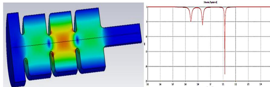
Fig. 3. CST Microwave Studio design of the C-band  $a/\lambda=0.105$  cavity: (Left) distribution of the electric field's magnitude (left), field concentration at center cell confirms  $\pi$ -mode; (Right) Reflection coefficient versus frequency, 3 modes are present in C-band
