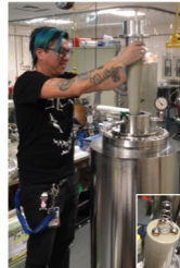
Postdoctoral fellow Gabriel Palacios-Serrano installing the modified epoxy receptacle to the SF 6 reservoir assembly on top of the testing chamber. Inset: Close-up view of the spring attached to the end of the epoxy receptacle.
