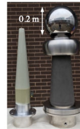
Picture of the tapered epoxy receptacle (left) next to the 500 kV doped alumina insulator with triple point junction shield and spherical test electrode.
