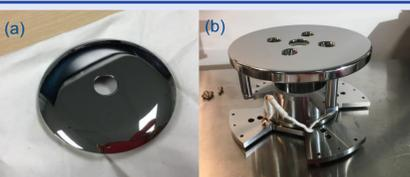
For the modified (flat) design: (a) front surface of the flat cathode that mates the spherical ball electrode and (b) the flat anode. The anode aperture (the hole at the center of the anode) is shifted by -1.6 mm vertically.
