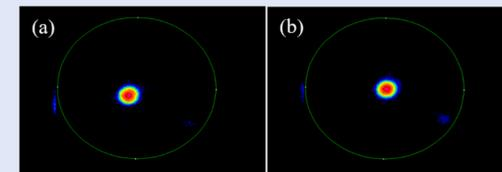
Electron beam for the redesigned photogun imaged on the first viewing screen 1 (a) with no beam steering, and, (b) beam centered on the first viewing screen with a very little steering by the first steering magnet set. For applied gun high voltage of -200 kV and laser spot of 0.35 mm rms size located at the center of the photocathode.
