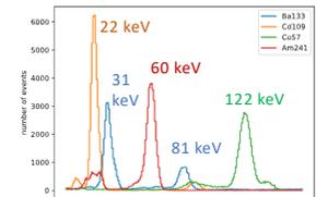
Spectra measured at UCSB with known calibration sources and the LaBr+PMT spectrometer.
