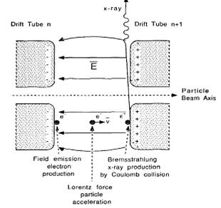
Diagram of Field Emission Electrons and resulting bremsstrahlung photons from [2].
