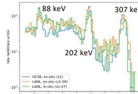
Scaled LYSO calibration spectra in-situ (at LANL DTL with background RF) and at ex-situ (labs at LANL and UCSB). The events are selected to have the <sup>176</sup>Lu gamma rays tagged by a coincident hit in the LYSO.
