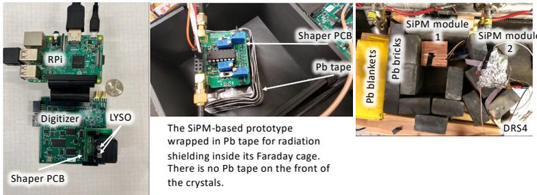
The SiPM-based prototype wrapped in Pb tape for radiation shielding inside its Faraday cage. There is no Pb tape on the front of the crystals.
