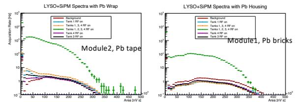
Scaled pulse area spectra (uncalibrated) for the LYSO+SiPM prototypes for different RF conditions.
