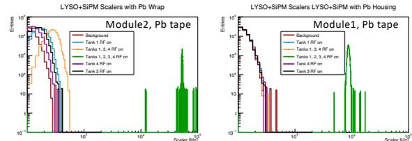
Hardware scalers (trigger rate without dead time) for the LYSO+SiPM modules in different RF conditions.
