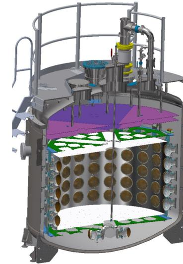
**CCM:** 10-ton Liquid Argon (LAr) detector instrumented with 200 8" Photo-multiplier tubes, veto region, shielding, fast electronics.
