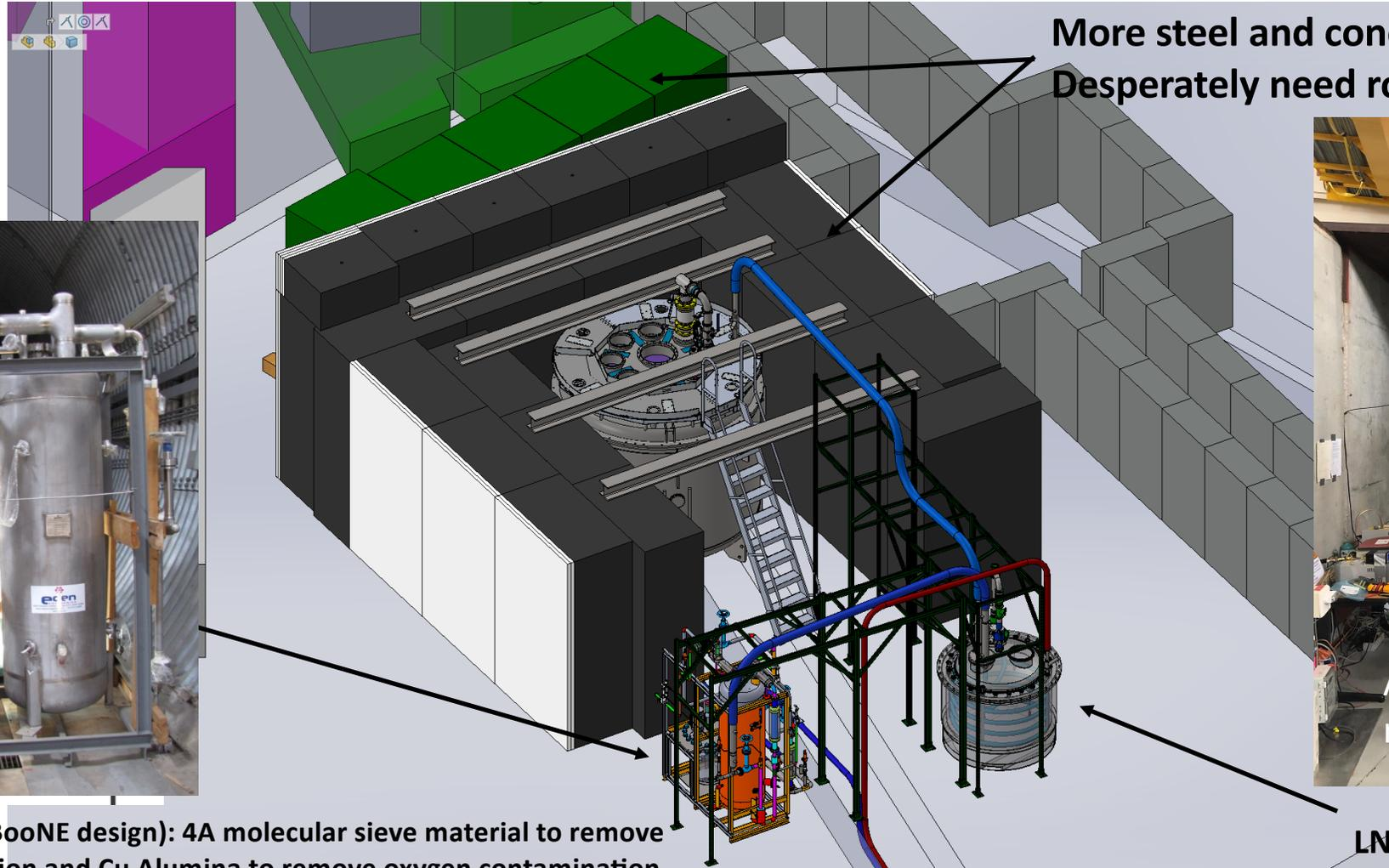
More steel and concrete shielding added.
