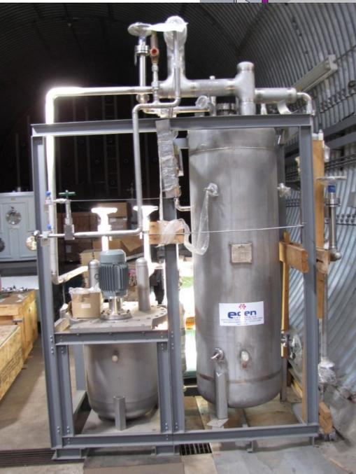
Filter skid (MicroBooNE design): 4A molecular sieve material to remove water contamination and Cu Alumina to remove oxygen contamination. LAr recirculation turn over time of ~three hours (see backup slide 50)
