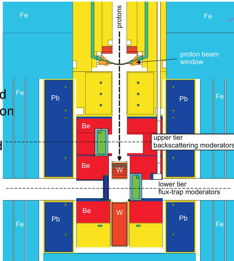
**Fig. 1.** Elevation view of the Lujan Center's TMRS geometry used in our calculations. The main components are labeled: split tungsten target (W), beryllium reflector (Be), lead reflector–shield (Pb), and the steel reflector–shield (Fe).
