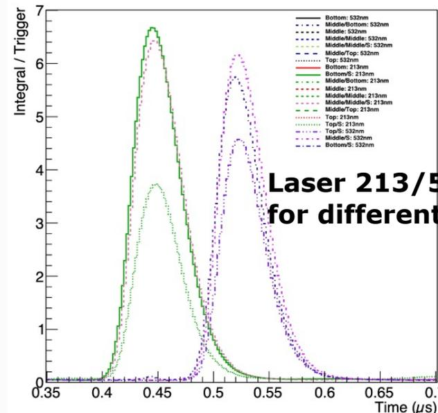
Laser 213/532 nm response for different path lengths
