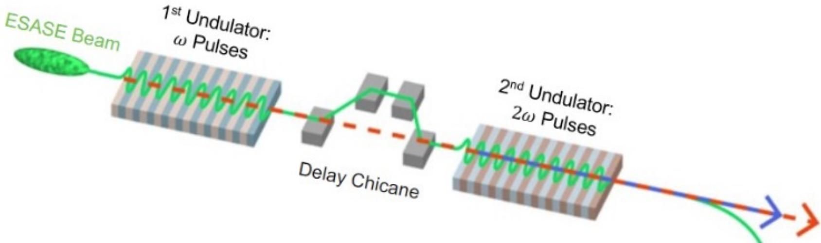
Minimal delay constrained by **the slippage of the 1<sup>st</sup> pulse in the 2<sup>nd</sup> undulator section**
