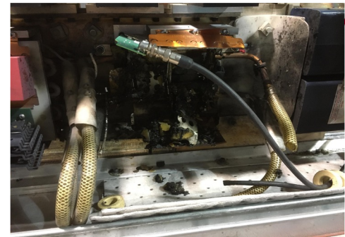
Transistor failure due to transformer saturation
