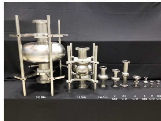
1-cell Fermilab cavities of various frequencies
