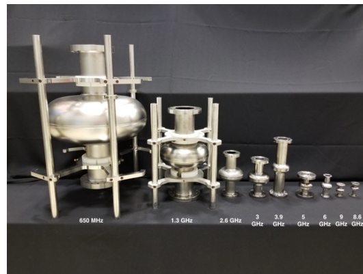
1-cell Fermilab cavities of various frequencies
