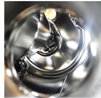
2022 refurbishment of 109 MHz (After electropolishing)
