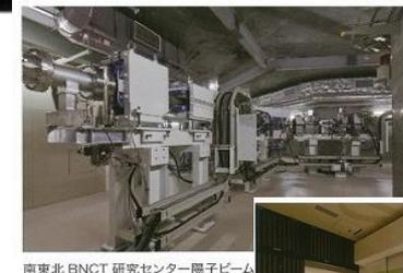
Cyclotron based BNCT at Fukushima
