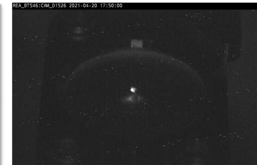
Viewer image in SECAR beamline, beam is < 1 mm
