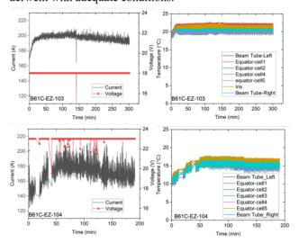
Figure 4: Current and cavity temperature profiles during EP of B61C-EZ-103 (top) and B61C-EZ-104 (bottom).
