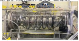
Figure 1: EP tool with a 650 MHz 5-cell cavity.
