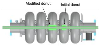
Figure 2: Schematic of the initial (cathode-A) and modified (cathode-B) cathode donuts, which were extended aluminum structure on the cathode pipe.
