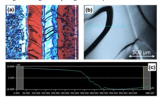
Figure 5: An equator surface of B61C-EZ-103 after the surface processing: (a) optical image, (b) confocal laser microscope image of the replica of the equator surface, and (c) surface profile along the line shown in (b).
