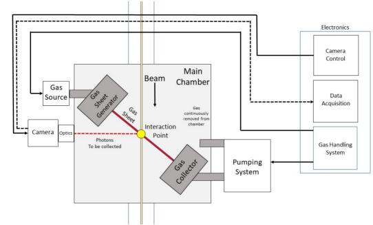
Figure 2: High-level overview of proposed system.
