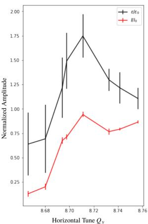
Figure 2: Saturated intensity and emittance of AGS experiments near resonance crossing. Growth seems consistent with that of high intensity bunched beam in SIS [1] including possible secondary resonance.
