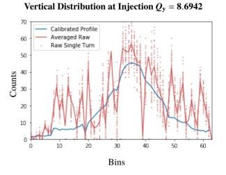
Figure 1: A vertical eIPM distribution taken at AGS injection. Raw profiles are in red, calibrated final profile is in blue. Any bins with obviously incorrect results are considered 'dead' and are removed from the data. Large tails are also observed, and are most likely overstated. Since this data is taken at injection, this is not due to the 3rd order resonance. Tails could be a calibration error or growth from the AGS Booster.
