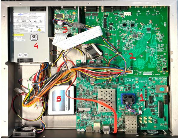
Figure 2: New LLRF controller chassis.
