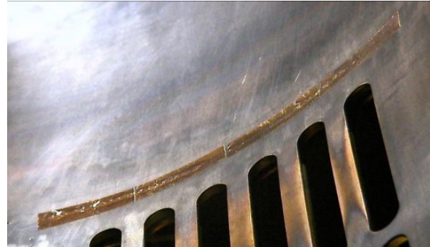
Figure 3: Blistered copper tape.
