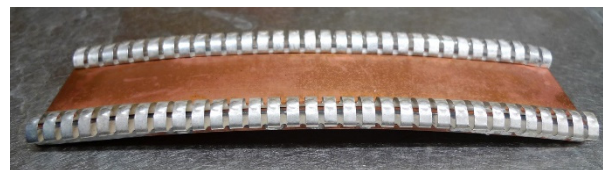
Figure 4: Finger stock brazed to copper bridge.
