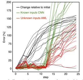
Figure 3: Error is shown in percent for each of the 15 projections of the beam's 6D phase space as the input beam distribution, charge, and solenoid strength are moved beyond the span of the training set.
