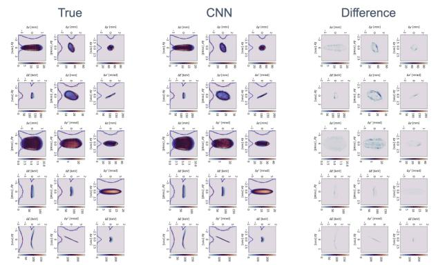
Figure 2: Projections of the beam's true 6D phase space are shown on the left, CNN predictions generated from the 2D latent space are shown in the middle, and the difference is shown on the right. Note that for each of the 15 projections the color scale of True, CNN, and Difference is the same.
