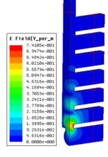
Figure 6: E-field structure of the operating eigenmode.
