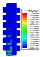
Figure 3: E-field structure of Bragg reflector at 10 GHz.
