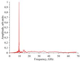
Figure 10: Fourier spectrum for the field excited in the PBG resonator.
