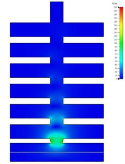
Figure 9: Instantaneous field distribution 10 ns after the bunch has passed.
