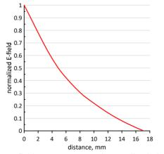
Figure 7:  $E_x$ -field component near the coupling hole across the beam line.
