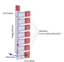
Figure 5: HFSS model for the open PBG resonator of OBPM.
