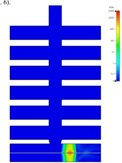
Figure 8: Instantaneous field when the bunch approaches to the resonator.
