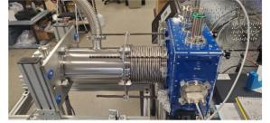
Figure 1: Vacuum envelope with the cryocooler and pumping port on the left and the (blue) instrumentation volume with feed-throughs on the right.
