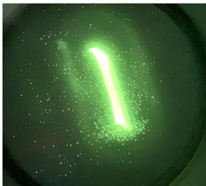
Figure 6: Raw measurement of first ions detected on ion microscope at the Pegasus lab, using laser-based ionization for commissioning.
