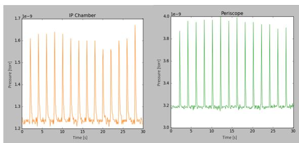
Figure 3: Measurement of vacuum levels during gas jet operation (0.5 Hz), attaining 1E-9 torr rapidly after pulse is evacuated.
