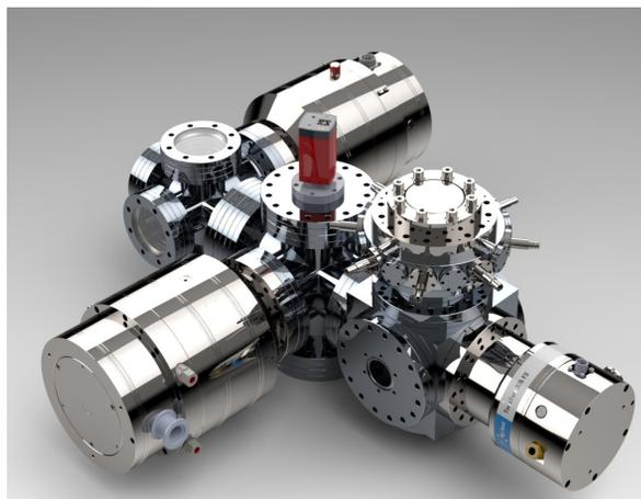
Figure 1: Rendering of gas sheet ionization monitor. The overall footprint of the monitor is < 1 m in the transverse direction, and < 200 mm in the longitudinal direction (i.e. beam axis).
