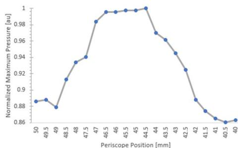
Figure 2: Measurement of gas density showing ~ 8 mm length, equivalent to long dimension of slotted skimmer.
