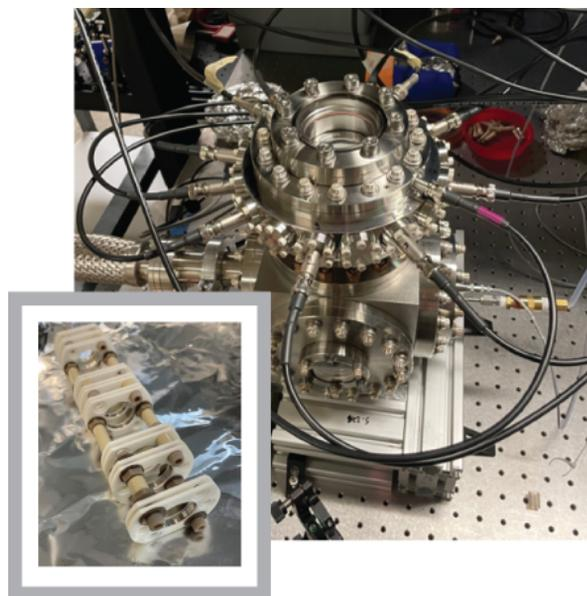
Figure 4: Photograph of the ion microscope chamber undergoing testing on the benchtop. The phosphor screen is visible at the top through a fused silica vacuum window. Inset: photograph of the electrostatic lens array during assembly.
