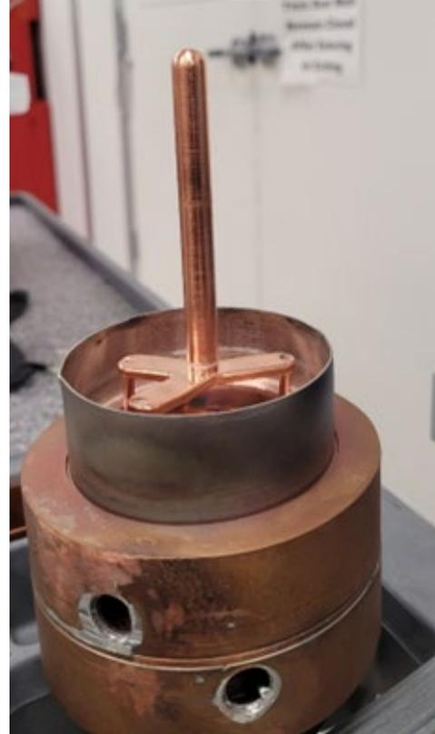
Figure 1: Photos show internal structure, ten cavities, straps and antenna attached to anode body. The new antenna design will have five legs.
