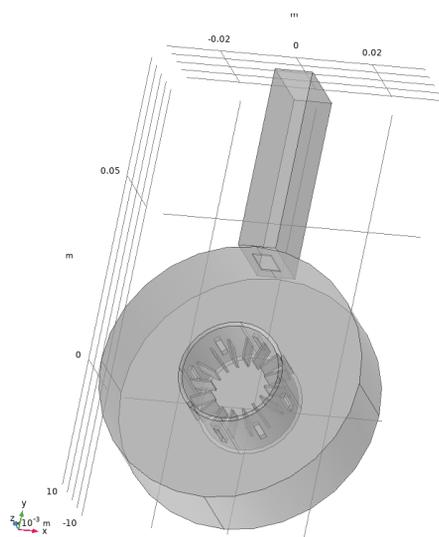
Figure 4: COMSOL model of a Coaxial Magnetron.
