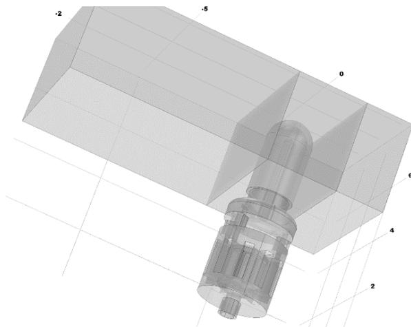
Figure 2: conventional coupling of the magnetron to a waveguide.
