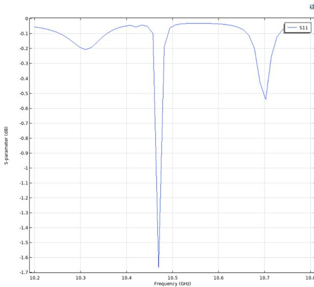
Figure 6: RF power output from co-axial magnetron showing that pi-mode is well separated from other modes.
