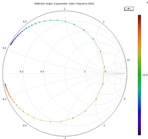
Figure 7: Smith Chart shows that coupling is  $\sim 5$ .
