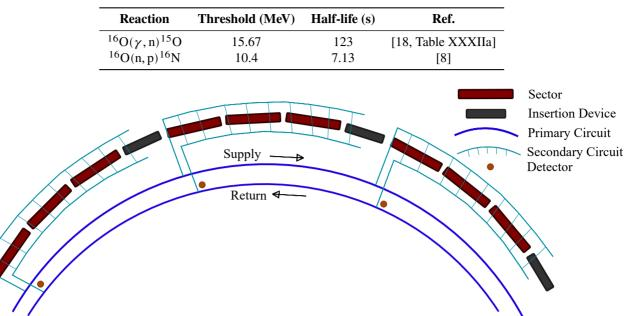
Figure 1: Schematic illustration of primary and secondary water systems. With approximately one secondary system per machine sector, detectors can be placed at each connection to the primary circuit to provide segmented coverage of the entire ring. Short flexible hoses supply and return water from individual accelerator and front-end components.
