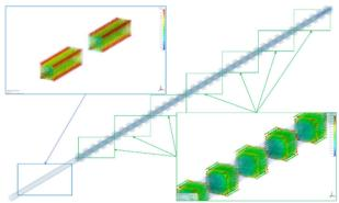
Figure 2: Calculation volume for PS runs. Insets show imported RF electric field (part; bottom) and magnetic field of the quadrupole doublet (top left). Thin blue and green arrow lines indicate locations of imported fields.
