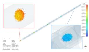
Figure 3: Snapshot of 5 bunches of 50K particles in M5T1 at t = 24 ns. Color indicates particle energy; the scale is on the right. Particles move from top right to bottom left.
