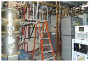
Figure 1: Old triode and tetrode RF amplifiers.
