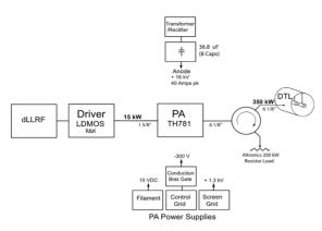
Figure 2: Diagram of New RF Amplifier System.
