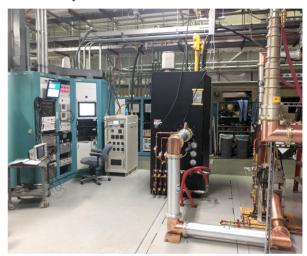
Figure 3: From left to right: LLRF, cRIO controller, SSA, PA (black unit), Circulator (end view) and Load (vertical).
