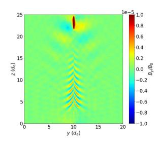
Figure 3: The field pattern of the plasma wave generated by the idealized bunched electron beam at a propagation distance of 362.1 m, represented by the distribution of  $B_y/B_0$ . The beam shown spans from  $z = 21.3 d_e$  to  $z = 25.0 d_e$ .
