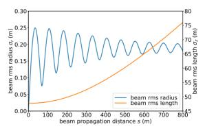
Figure 1: Evolution of the rms radius and the rms beam length of the simulated pulsed electron beam generated by the Beam-PIE experiment as it propagates parallel to the background magnetic field.
