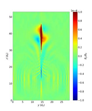
Figure 2: The field pattern of the plasma wave generated by the Beam-PIE electron beam at a propagation distance of 504.5 m, represented by the distribution of  $B_y/B_0$ . The beam shown spans from  $z = 22.6 d_e$  to  $z = 46.5 d_e$ .
