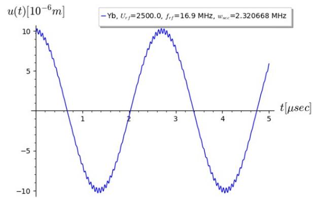
Figure 2: Secular motion is determined by the particles trajectory influenced by the rf focusing fields. Micromotion is a result of the trap rf frequency and the particle large amplitude away from the center of the symmetric fields.
