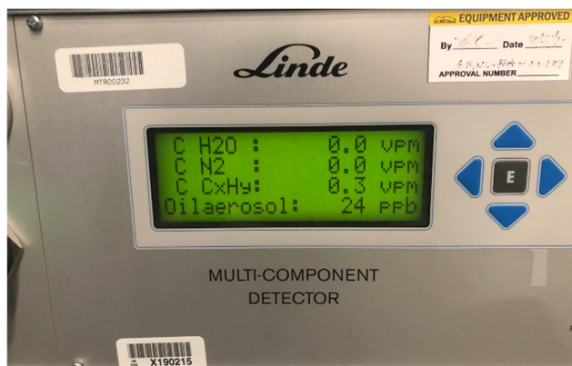
Figure 5: LINDE analyzer readings during sampling from inlet of CMS oil purification carbon bed.
