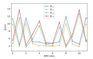
Figure 5: Measured Ripken Twiss parameters for one supercell (cell 30 and 1). Here the round beam was obtained at the short straight section between BPM 5 and 6.
