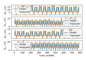
Figure 3: Comparison of the Ripken Twiss functions between the lattice model and the extraction from simulated TbT data.
