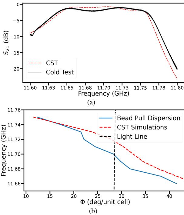
Figure 6: (a) Comparison of the  $S_{21}$  parameter from the cold test and from simulations. (b) Comparison of the dispersion curve from the bead pull test and from simulation. The dotted black line represents the dispersion curve for light (relativist electron beam).
