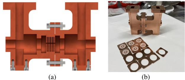
Figure 4: (a) Mechanical drawing of the MTM structure. (b) Fully-assembled structure (and spare plates for display).
