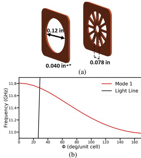
Figure 1: (a) Unit cell of the MTM accelerating structure. (b) Dispersion curve for the fundamental  $\text{TM}_{01}$ -like mode of the optimized unit cell.
