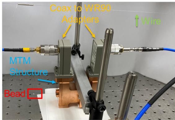
Figure 5: Experimental setup for cold test.
