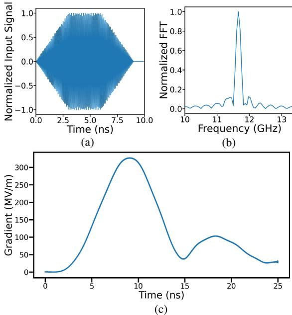
Figure 2: (a) Normalized input pulse (voltage signal) for the MTM structure, as extracted from the metallic PETS. (b) Normalized frequency spectrum of the input pulse. (c) Gradient from a probe at the center of the structure, when the peak power from the input pulse is 500 MW.
