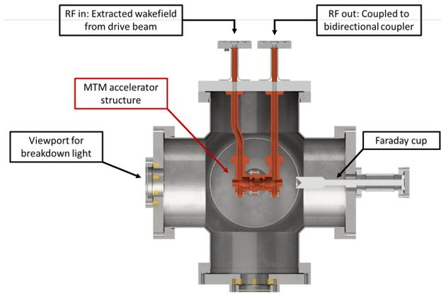
Figure 7: Schematic for a future high power test at AWA on the MTM accelerating structure.
