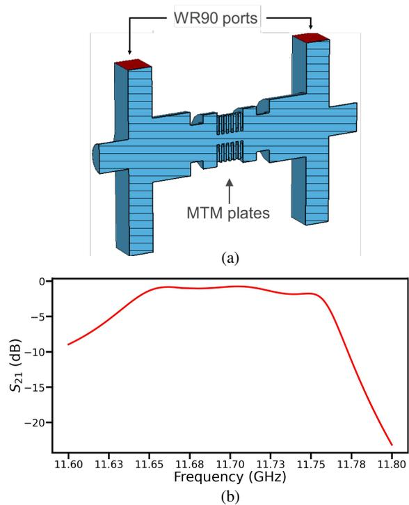
Figure 3: (a) Vacuum model of the 6-cell periodic MTM accelerating structure with couplers. (b) Simulated  $S_{21}$  parameter from CST frequency domain simulations.
